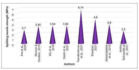
Figure 11. Maximum splitting tensile strength results after 28 days from different studies
